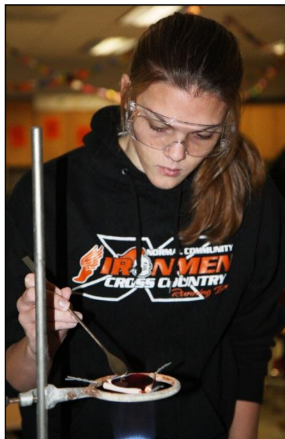
Figure 7.8: (Left) A student creates a Schottky diode. (Right) A student tests the diode to check that its current conducts in only one direction.
