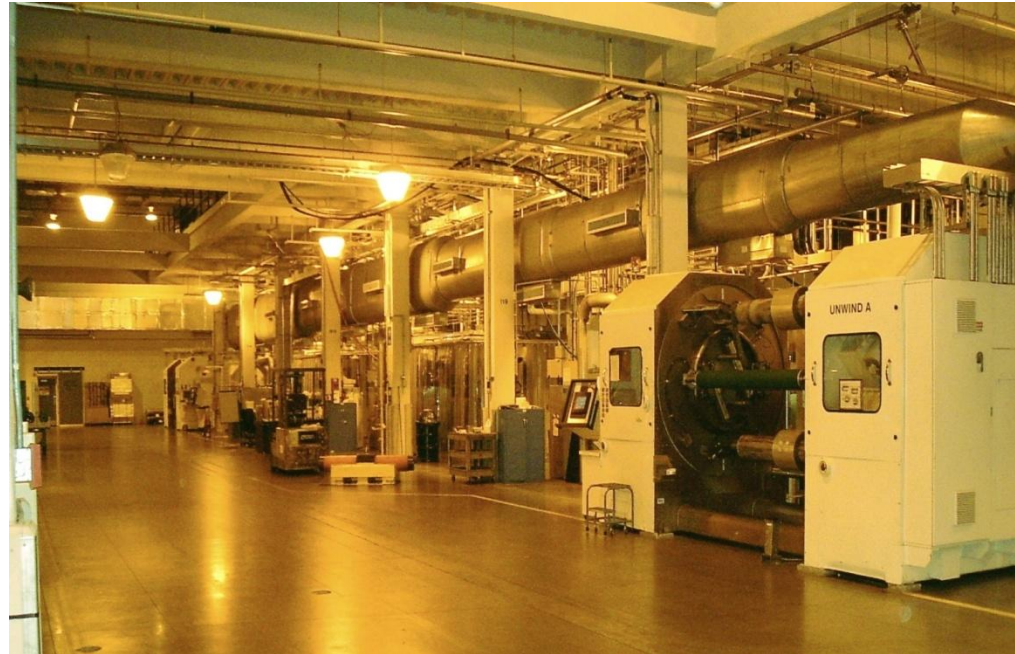
Roll-to-roll manufacturing of plastic solar modules at Konarka facility in New Bedford, MA
