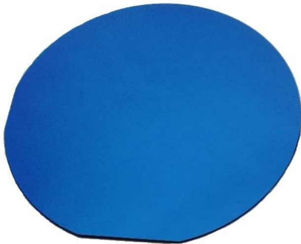
100 nm Al 2 O 3 coating on Si wafer
