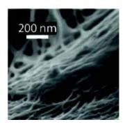
Recently, Schoen et. al. investigated the incorporation of silver nanowires (AgNWs) and carbon nanotubes (CNTs) within a matrix of cotton, enabling a membrane with multiscale nanostructured
